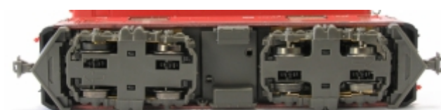
Complex conversion from 9mm (left) to 6.5mm (right).
